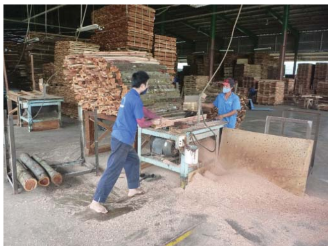
Modern wood processing industries can operate at small scale: Sawing small diameter acacia logs in Vietnam (Credit: C. Harwood)
