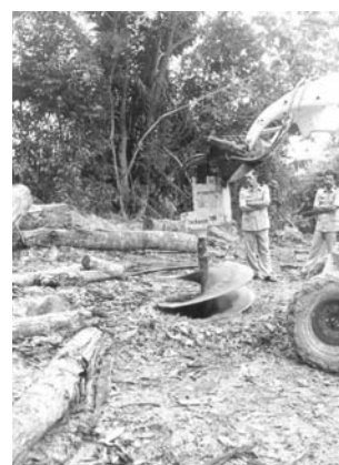
FIGURE 7 Planting of seedlings using a big hole has been more successful with help from a Skid Steer Loader
