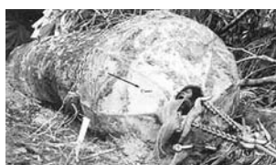
FIGURE 6 Log-hauling process using a cone, commonly known as ‘Ecolog,’ aims at minimizing damage to the environment
