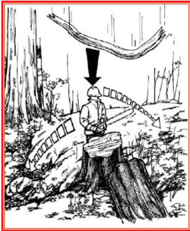
Fig. 1: Safety risks associated with tree felling. Falling branches from above (window-makers; left image) poses a severe risk to tree fellers especially when tree crowns are intertwined. Tree kickback (right image) is associated with poor cutting techniques and is most common when the backcut is lower than the directional notch.
