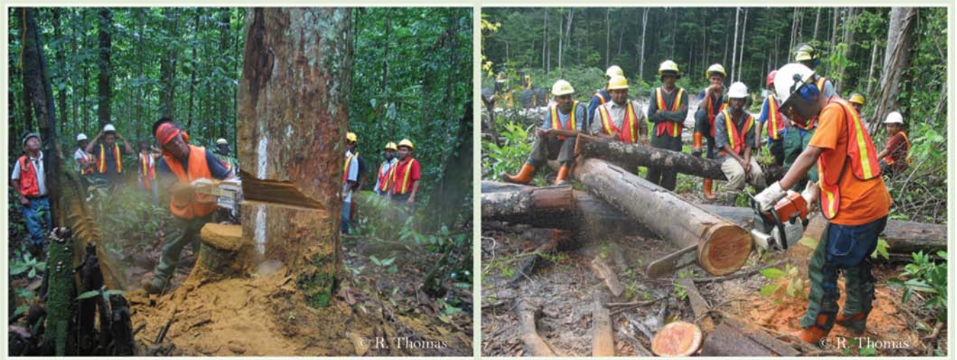
Fig. 3: Trainers at the Forestry Training Centre (FTCI) located in Guyana demonstrate directional felling techniques (left) and good bucking practices (right) to forestry workers. Note use of personal protective equipment.
