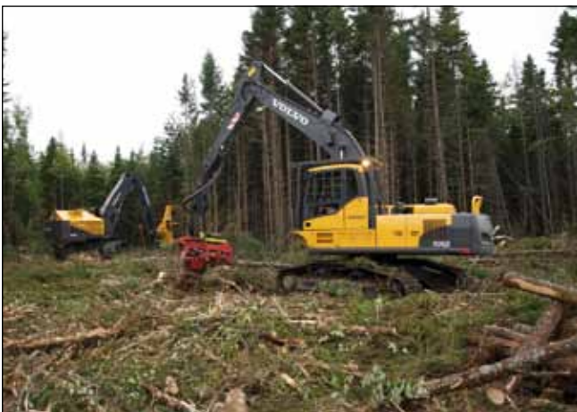
Perfect partners – a Volvo tracked harvester and (background), one of the latest feller bunchers, which can also be equipped with a harvester head, for added versatility.
