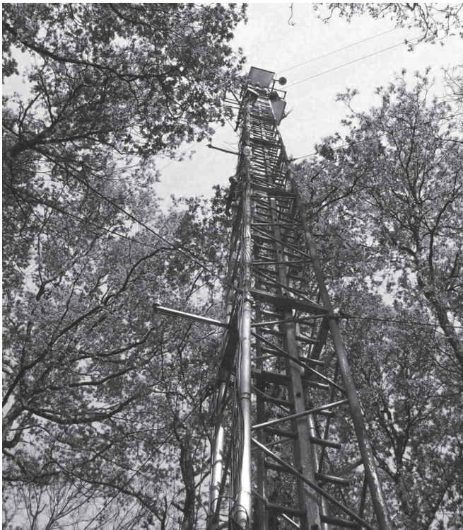
The flux tower at Alice Holt Research Forest monitors the exchange of carbon dioxide between the atmosphere and the surrounding forest.
